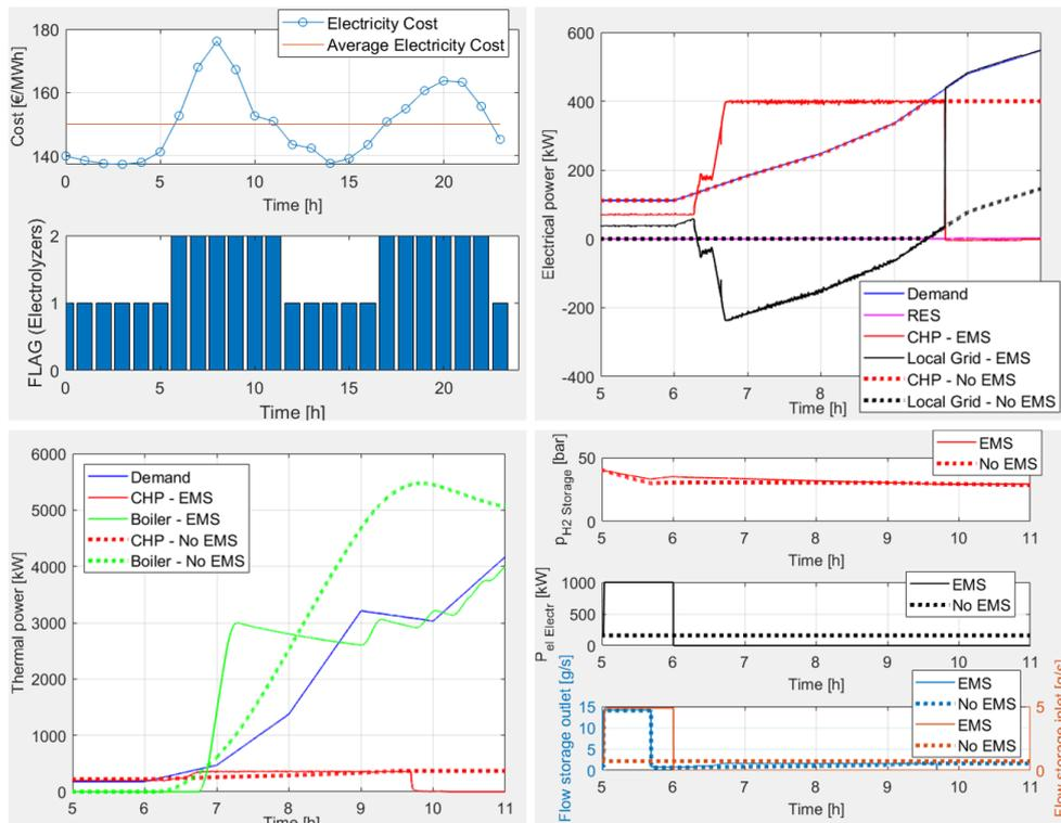
Figure 6 - Electrical costs, demands and preliminary results for tests in cyber-physical mode against simulations with a standard management approach, as described in [11] or In D3.3.
