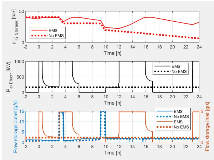
Figure 12 - 26-hour test with 80 €/MWh for the syngas cost: hydrogen generation and storage.
