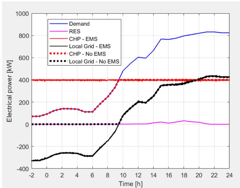
Figure 13 - 26-hour test with 5 €/MWh for the syngas cost: electrical power.
