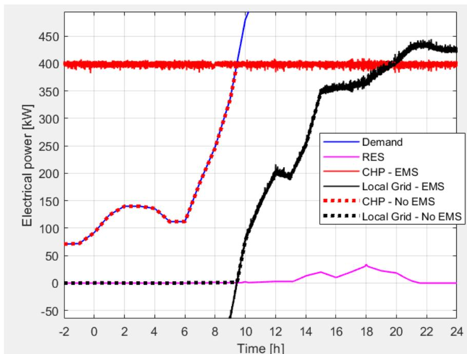
Figure 14 - 26-hour test with 5 €/MWh for the syngas cost: electrical power (zoomed plot).
