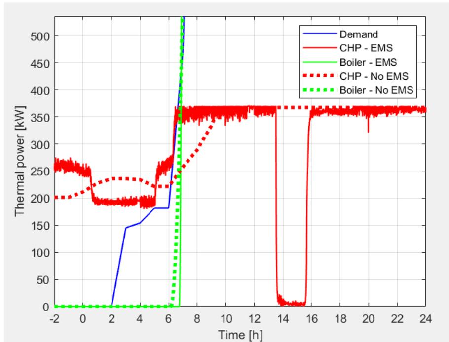
Figure 11 - 26-hour test with 80 €/MWh for the syngas cost: thermal power (zoomed plot).
