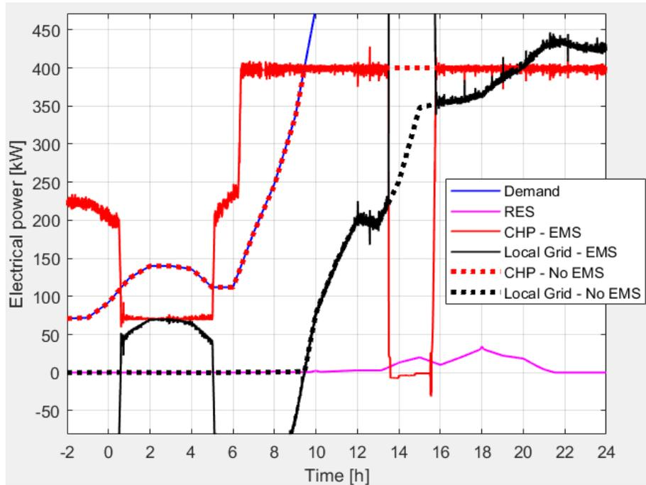
Figure 9 – 26-hour test with 80 €/MWh for the syngas cost: electrical power (zoomed plot).
