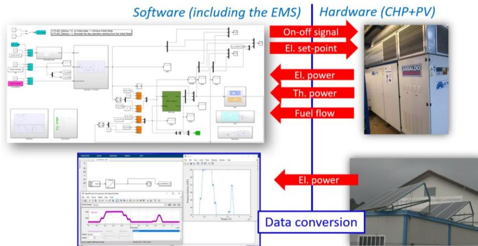
Figure 5 – Data communication between the software and the hardware (tests in cyber-physical mode).
