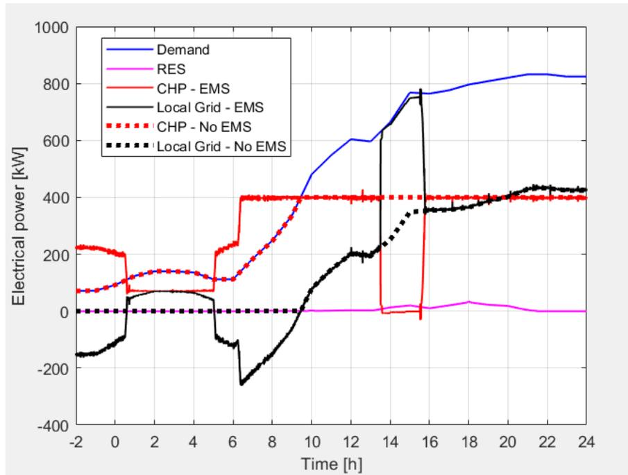
Figure 8 – 26-hour test with 80 €/MWh for the syngas cost: electrical power.
