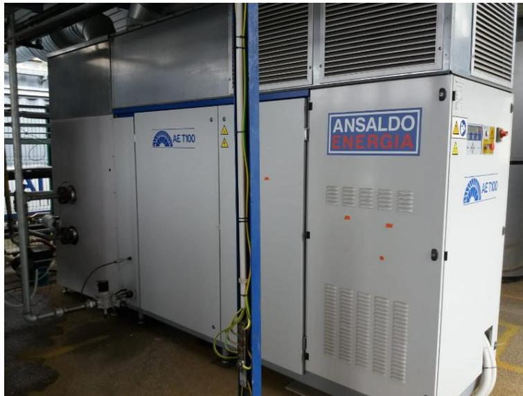
Figure 1 - AE-T100NG microturbine in the UNIGE laboratory.
