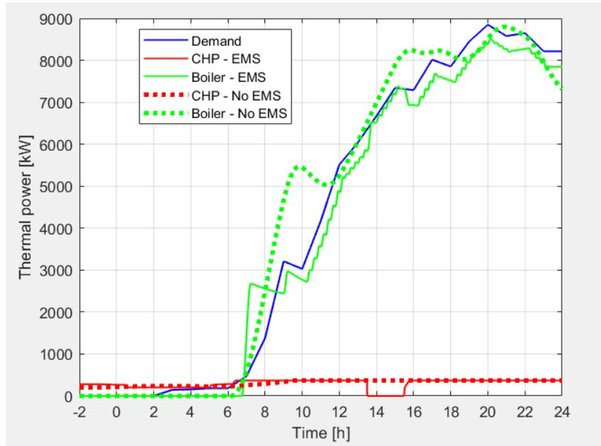
Figure 10 - 26-hour test with 80 €/MWh for the syngas cost: thermal power.
