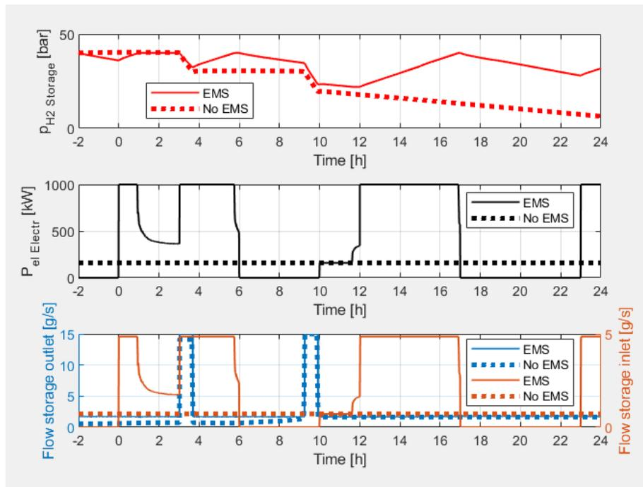
Figure 16 - 26-hour test with 5 €/MWh for the syngas cost: hydrogen generation and storage.
