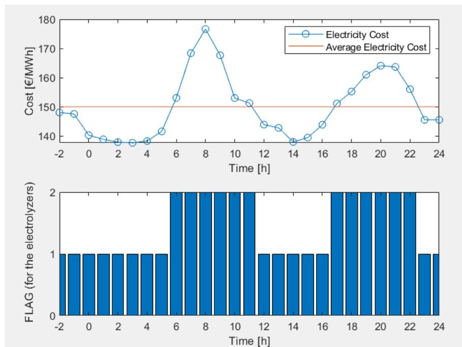
Figure 7 - Electricity cost (hour-by-hour trend and average value) and the flag for the electrolyzers.
