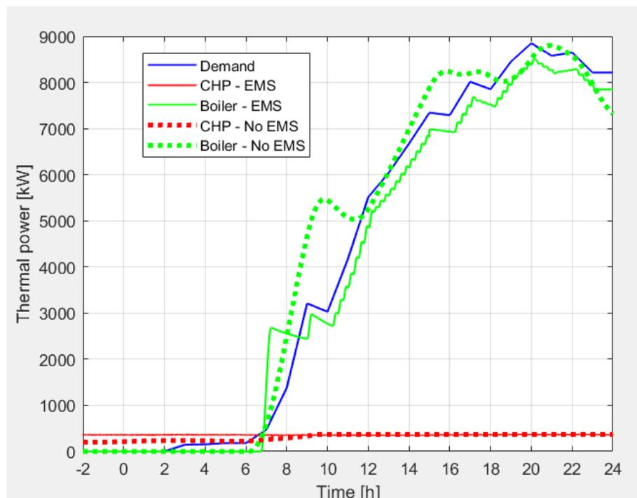
Figure 15 - 26-hour test with 5 €/MWh for the syngas cost: thermal power.
